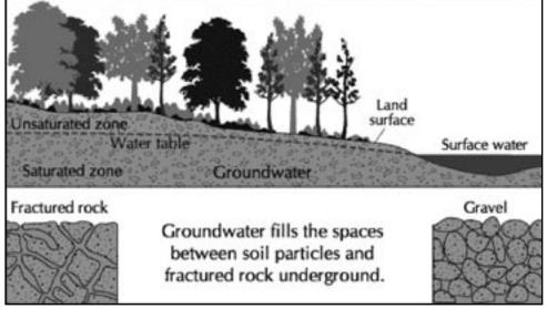
Figure 1. Image courtesy of the US Geological Survey, adapted by the Groundwater Foundation.
